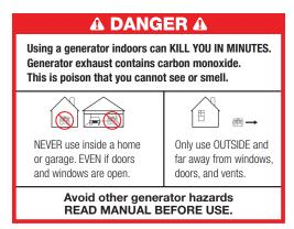
Generator exhaust contains high levels of carbon monoxide (CO), a poisonous gas you cannot see or smell. If you can smell the generator exhaust you are breathing CO. Even if you cannot smell the exhaust, you could be breathing CO.
